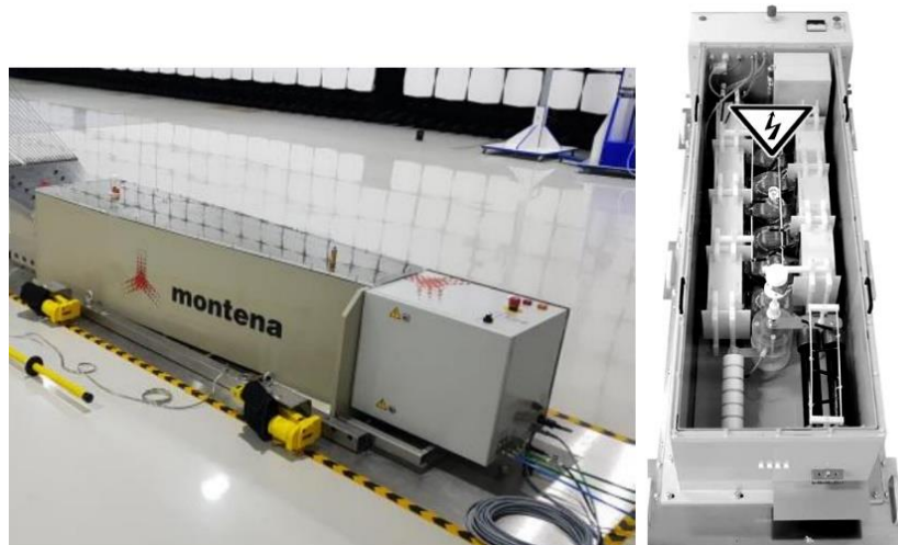
Fig. 6. Compact PVG, manufactured by the company Montena.
