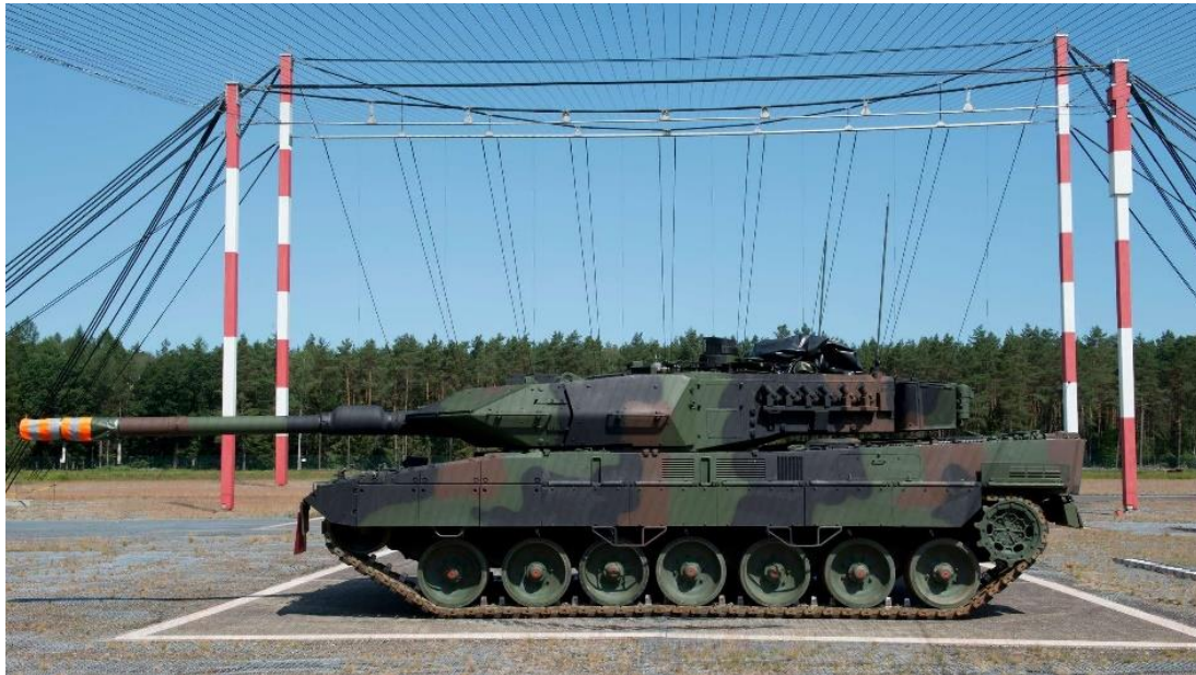
Fig. 8. A battle tank mounted on a HEMP test stand.
